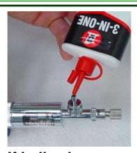
If ball valves are sticking, add some oil or silicone, and press trigger several times.
