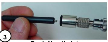
Push Needle into "Push to Connect" (PTC) fitting
