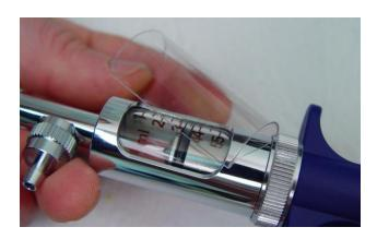
**Use plastic guard to protect Glass Barrel - 975-9446**
